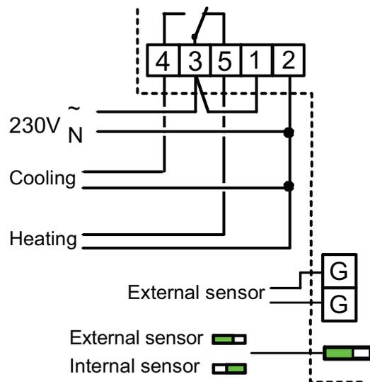
NB The thermostat can control either cooling or heating, but not both simultaneously.
