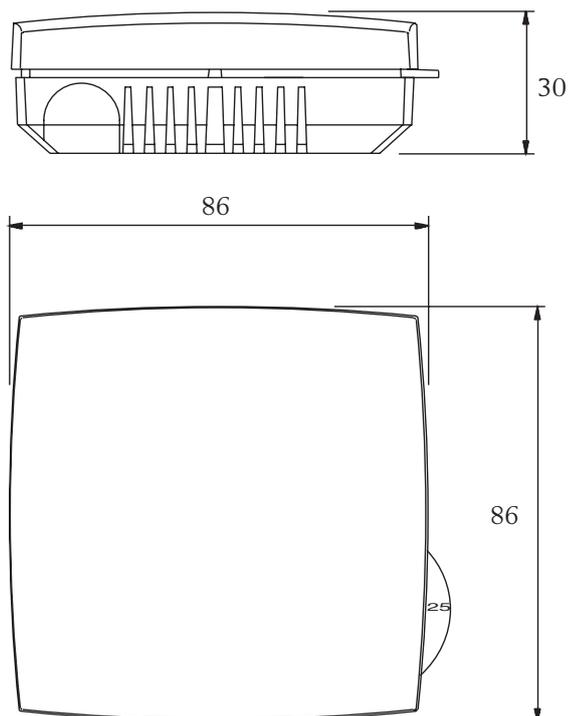
Measurements in mm unless otherwise specified.
