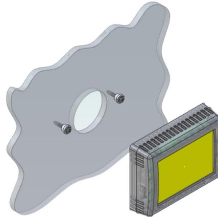
**Step 4:** Remove mounting tab before mounting on the wall.
