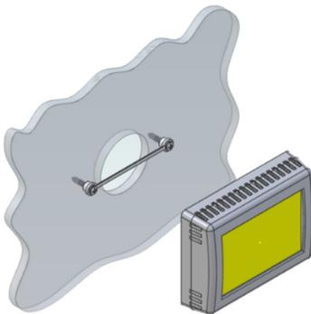
**Step 3:** Screw in second screw making sure the two buttons remain level.
