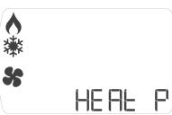
**NOTE:** If you have a heat pump system, press the center button to select. CS1 will now ask you to confirm your valve type. Use the up and down arrows to toggle between O & B Valves, press the center button to select:
