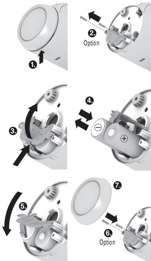
1. Pull off the adjustment dial. To do so, start at the notch on the bottom of the device.
