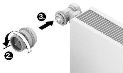
2. Turn the adjustment dial of the valve baseplate counter-clockwise until it stops.
