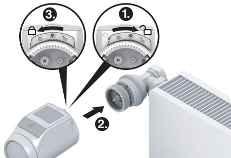
1. Ensure that the slide on the radiator controller is in the open position.
