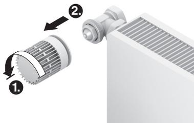
1. Turn the old thermostat head counter-clockwise until it stops and loosen the mounting ring.
