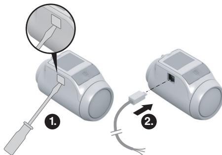
1. Remove the side cover from the radiator controller.
