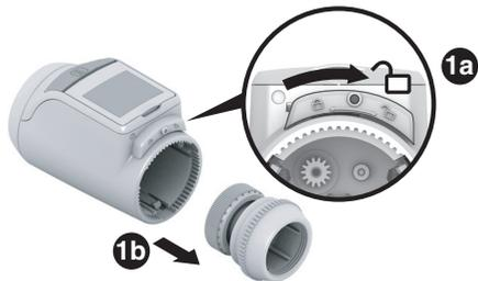
1. Separate the valve baseplate from the radiator controller. To do so, push the slide towards
