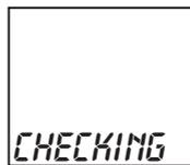
*The radiator controller is ready to receive radio signals from the central operating device.*
