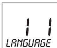
The right-hand digit shows the current setting. The parameter is displayed additionally in plain text. For example, the display **1 1** stands for Parameter 1 (language) with Setting 1 (German).
