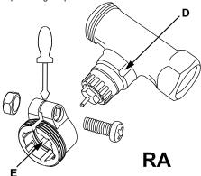
During installation, please ensure that the pins inside the adapter (E) are lined up with the notches (D) on the valve. Ensure that a suitable adapter for the valve is properly clipped on.
