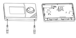
As shown in the picture above, press the screwdriver forward from the space shown, bend the tabs and separate the front cover. Insert 2 new AAA alkaline batteries in the battery housing with the correct battery direction. Replace both batteries at the same time. Then align the front part of your Room Thermostat to the back and squeeze it towards the back
