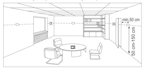
If the room thermostat is to be used with the wall bracket, the wall bracket must be mounted on a flat wall.
