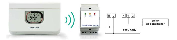
With one Intellitherm C58RF can be controlled more CH173D actuators.
