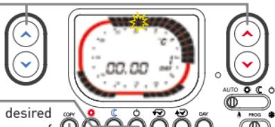
Move the switches to the AUTO and PROG positions to start the program setting. The display will show time 00.00 and DAY1.
