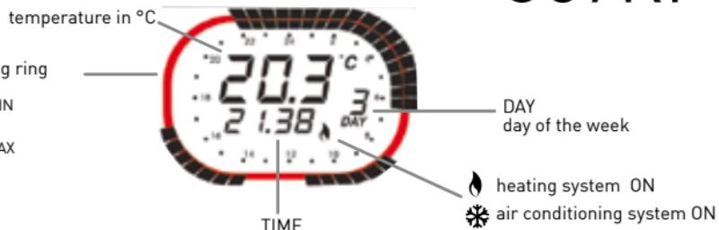
The program setting ring shows a 24-hours clock, divided into 30 min sectors. The sector colour indicates the set temperature for that period.
