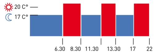
STANDARD AUTOMATIC PROGRAMS WITH THE TIME AND TEMPERATURE ALREADY PROGRAMMED AT THE FACTORY.
