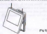
5. Connect the control board and back cover.
