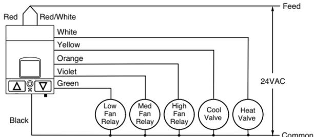
**Figure C - Installation - 2-Pipe Fan Coil with Aquastat Configuration**
