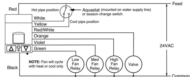
**Figure D - Installation - 2-Pipe Fan Coil with Electric Heat Configuration**
