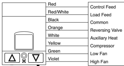
**Figure B - Installation - 4-Pipe Fan Coil Configuration**
