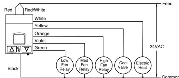
**Figure E - Disable HVAC Unit when Existing Light Circuit is Turned Off**
