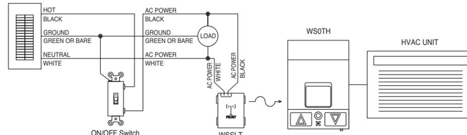
**Figure F - Key Card Switch Control of Thermostat**
