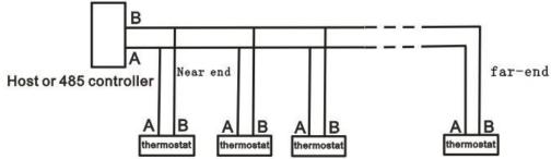
When 485 communication distance is more than 300m, need to increase terminal resistance in 485 the beginning of the communication terminal and end. Especially, if communication equipment quantity is less in trunk(less than 22pcs). When increase terminal resistance, only short circuit the terminal resistance jumper J5 of thermostat.
