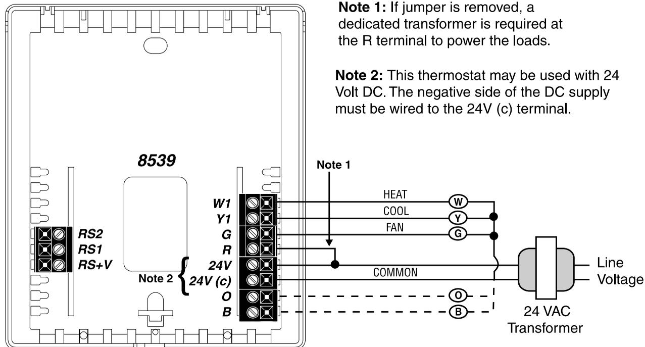
**Note 1:** If jumper is removed, a dedicated transformer is required at the R terminal to power the loads.
