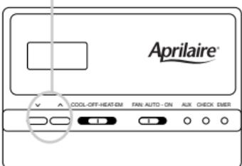
2. Press either the **▼** or **▲** button to adjust the temperature differential up or down.
