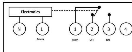
Note: The switch is volt free. Com should be linked to L for mains switching.
