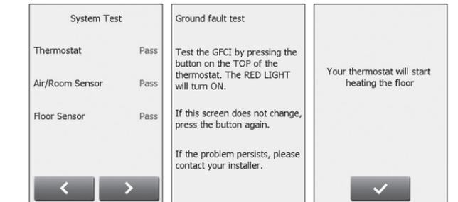
Perform the system and GFCI tests. Once the thermostat setup is complete, confirm "Your thermostat will start heating the floor" to complete the startup wizard.
