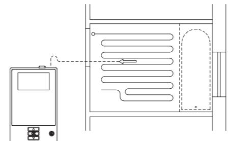
The floor sensor is recommended placed in an non conductive installation pipe, which is embedded in the floor. The pipe must be sealed in the end and placed as high as possible in the concrete layer. The floor sensor must be centered in between the heating cable. The power supply voltage must match the voltage rating of the heating cable.
