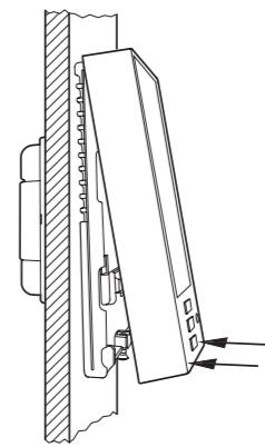
Remount the faceplate. Tighten the screw at the bottom. Perform GFCI/EGFPD test.
