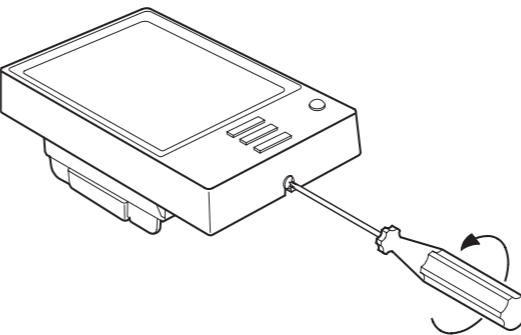
Loosen the screw at the bottom and remove the faceplate. Do not attempt to remove the screw completely.
