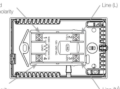
Turn power source OFF at breaker panel. Connect power supply wires to line side and heating cable wiring to load side of power base.
