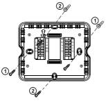
For vertical mount put one screw on the top and one screw on the bottom.
