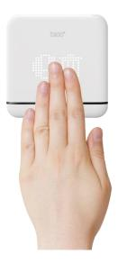
Touch the main display to reset the device back to factory settings. The exclamation mark and trash can symbol will blink to confirm the successful reset.
