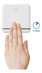
This will open the reset menu and the device will show a screwdriver and wrench symbol.
