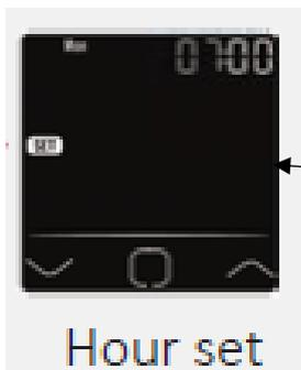
This section allows the hour to be changed. The hour can be changed by pressing the up and down arrow. When the right minutes have been selected press the middle button.
