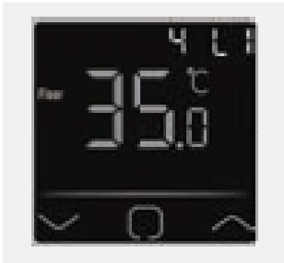
Select a temperature limit as this is needed to protect the floor.
