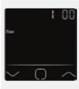
**00 => Floor Sensor:** run by floor sensor(default)
