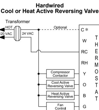
\* Common wire connection optional with batteries installed.
