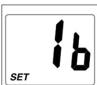
To exit configuration mode, press both the **LEFT** and **RIGHT** switches for 2 seconds or slide the mode switch to heat or cool.
