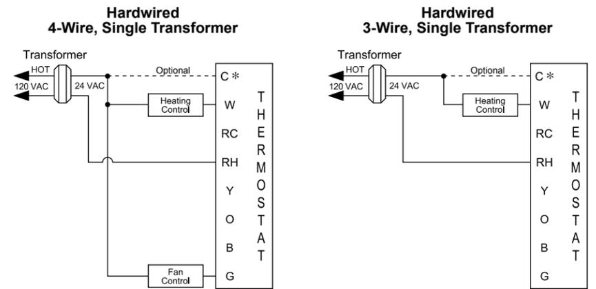
\* Common wire connection optional with batteries installed.
