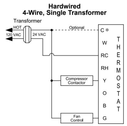
\* Common wire connection optional with batteries installed.
