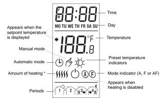
\* The thermostat displays the amount of heating required to maintain the desired temperature. For example, \$\int\_{\mathfrak{I}}\$ is displayed when heating is at 40 percent.
