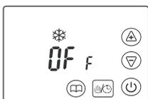
This indicates that the thermostat is in Frost Protection Mode
