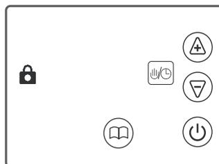
To unlock the screen, press and hold and simultaneously until the symbol is no longer displayed (approx 7 secs).
