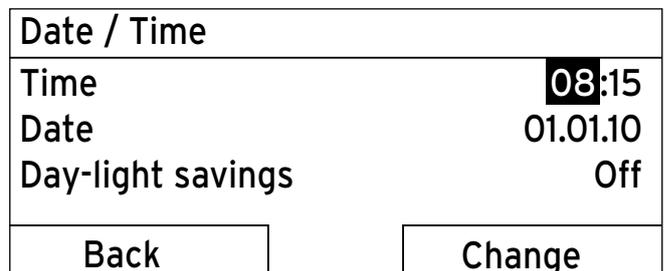
Fig. 4.7 Setting level: figure for hours is highlighted
