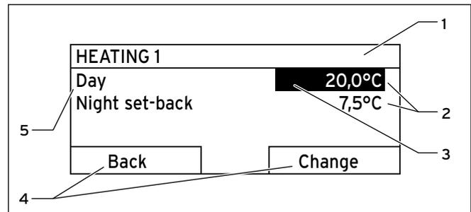
**Fig. 3.6** Display fields in the setting level
