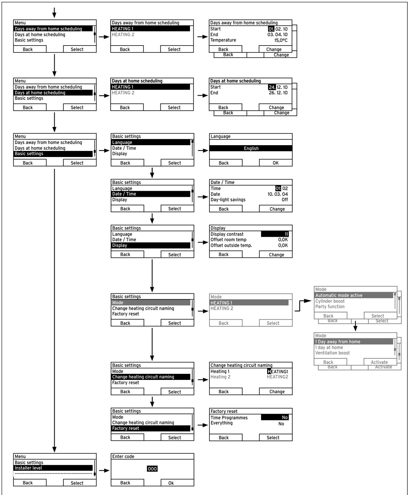
Fig. 4.11 Overview of the menu structure Part 2
