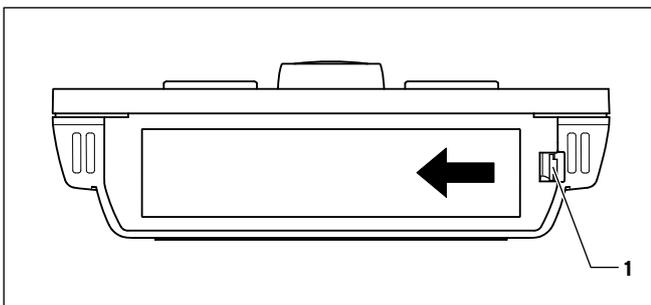
**Fig. 6.5 Opening the battery compartment**
