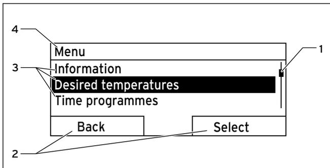
**Fig. 3.5** Display fields in the selection levels
