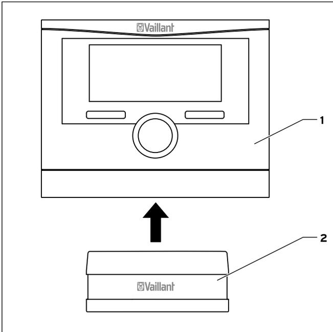
**Fig. 6.4 Removing the VRC 470f**
