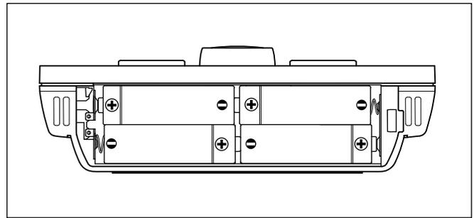
**Fig. 6.6 Layout and polarity of batteries**
