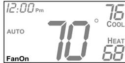
**Fan On** indicates constant fan operation. You may turn the fan on even if the thermostat is in the **Off** mode. Pressing the FAN button toggles this feature on or off.
