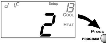
Press the **PROGRAM** button to leave the Setup screens. If no buttons are pressed, the display will leave the setup screens after 30 seconds.
