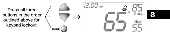
To **unlock** the keypad, press and hold the MODE button. While holding the MODE button, press the UP and DOWN buttons together. The
