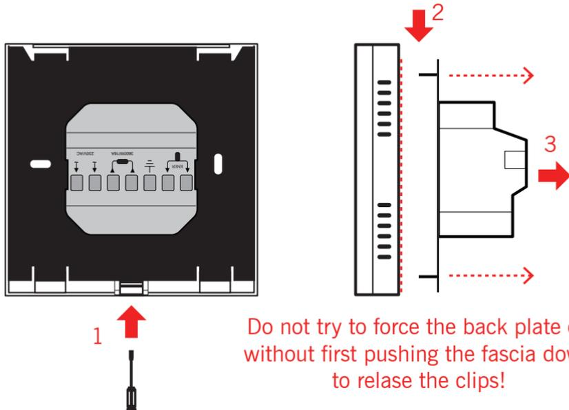
Do not try to force the back plate off without first pushing the fascia down to release the clips!
