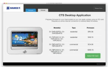
Every time the user runs the CTS Desktop App software, it automatically connects to the Source 1 Color Display website in the background and updates the software and firmware (the operating system for touch screen) at no cost.
