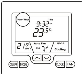
Your commercial programmable thermostat is able to be programmed by you, to automatically control the desired office heating and cooling temperatures.
