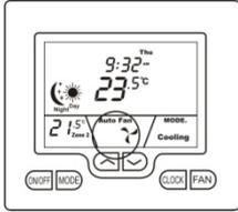
If your air conditioning system has one fan speed, your SMT-700 thermostat will display the fan information shown on the picture to the left. The words “High”, “Med” or “Low” will be absent from the LCD.
