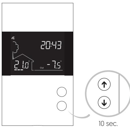
Get the setpoint to its minimum and hold the **down** button for 10 seconds to access the menu.
