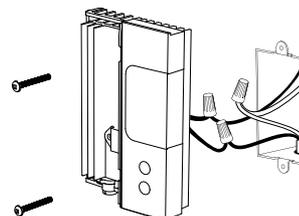
Make sure to firmly tighten the wire connectors for a secure connection. A loose connection can be a fire hazard.
