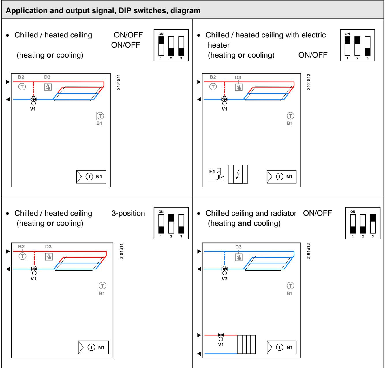
V1 Heating or heating / cooling valve actuator
