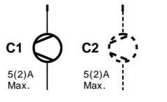
1-stage compressor and electric heater
