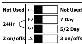
DIP Switches Shown in Factory Default Positions. (black = raised actuator of switch)
