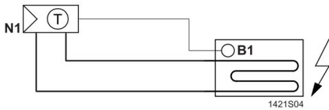
Room thermostat for control of electric floor heating systems. Floor temperature limitation with cable temperature sensor
