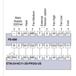
Note: In case of 220Vac systems, the PS-600 must be used. All outputs - 220Vac, 1A each (max)
