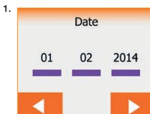
When the system has been installed and turned on for the first time, or after you have performed a factory reset, you must set the Date, Time and Floor Type. The thermostat will automatically guide you through the process.
