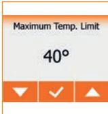
5. Use the **Up** or **Down** arrows to set the Minimum and Maximum Temp. Scales Confirm each setting with **✓**
