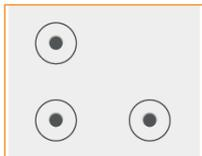
• Three circles containing dots are displayed on the screen; the thermostat cannot be operated. The thermostat is in **Screen Lock** mode. See “**Screen Lock**” on page 23 of this manual for instructions on how to unlock it.
