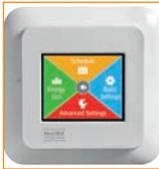
The **Open Window** function prompts the thermostat to detect an open window or door, by registering a rapid drop in temperature. With this function enabled, the thermostat shuts off the heating for 30 minutes to avoid needlessly heating a room and wasting heat.
