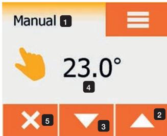
You can use **Manual** to override the current schedule and maintain a specified temperature around the clock. The thermostat will continue to operate in **Manual Mode** until you return to the heating schedule.
