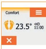
While in Comfort mode an X is shown on the home screen. Press this button to return the thermostat to heating schedule.
