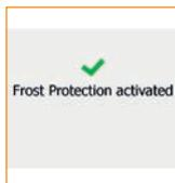
**Frost Protection** mode is used when heating is not needed but the temperature must be kept above freezing until changed manually. This is usually used in holiday cottages, outbuildings or similar properties that may be left unattended for long periods of time in the winter.
