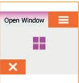
6. The home screen is replaced by the **Open Window** screen with a purple window icon if the thermostat detects a rapid drop in temperature
