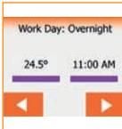
3. Press the **Work temperature**, if you want to change it, then press the **Up Arrow** or **Down Arrow** to set the temperature. Confirm with ✓ icon
