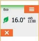
Eco Mode reduces the energy spent on unnecessary heating if you leave the room or house temporarily during a scheduled heating event. If you are going to bed early at 9pm, but your heating normally stays on until 11pm, pressing the Eco button will prevent the system heating needlessly for two hours.
