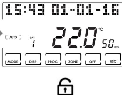
**NOTE:** with the **KEY LOCK WITH PASSWORD** function, the CH120RF keys connected to the MASTER CH180RF are also locked.
