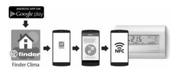
After downloading the APP, DO NOT move the smartphone away from the unit while communicating with/programming the thermostat.
