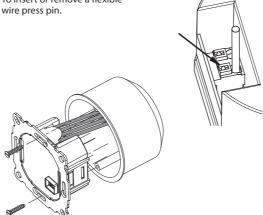
The plastic tab must be in place to provide insulation between the terminals/wires and the mounting screw.
