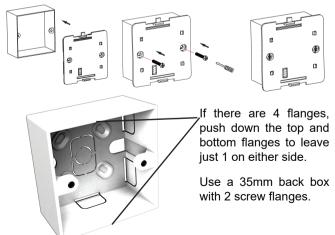
Route the wires through the back of the wall plate. Fit the wires to the wall-plate in accordance with the relevant diagram and in accordance with I.E.E. regulations.
