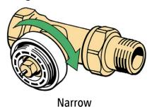
(5) Now, screw the Home Control Radiator Thermostat to the adapter ring installed on the radiator and tighten it hand-tight by rotating clockwise, applying gentle pressure.
