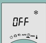
If the screen displays "OFF", your product is connected to the Tydom app (menu 1-10 = 1). The date and time details are no longer show on the thermostat screen.
