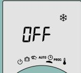
If the screen displays "OFF", your product is connected to the Tydom app (menu 1-10 = 1). The date and time details are no longer show on the thermostat screen.
