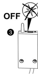
3 Make sure that the receiver LED has stopped flashing.
