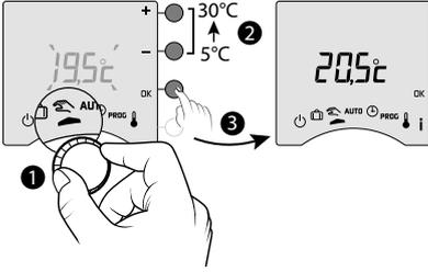
This mode is used to set a constant temperature (5 to 30°C)
