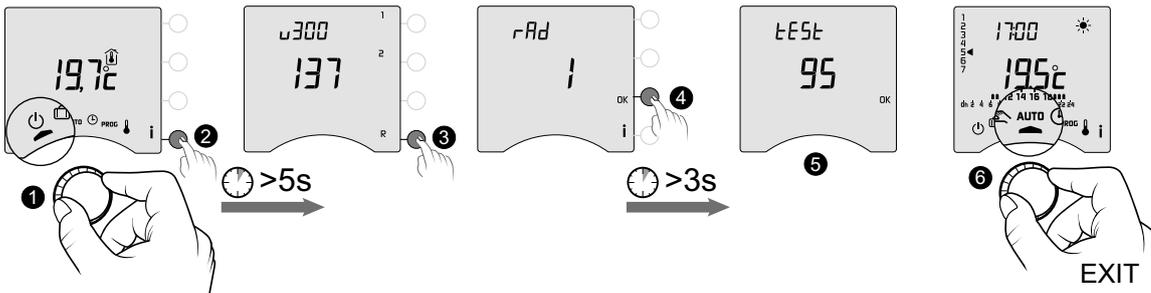
① Turn the dial on the transmitter to
