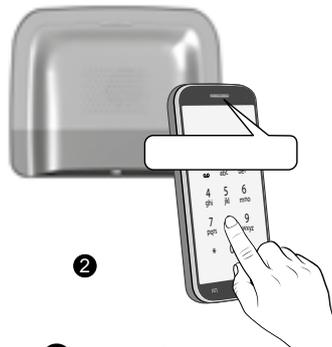
2 From the transmitter's main menu, tap #400, then tap 1: the transmitter announces "Configuration in progress..." and indicates the number of connected receivers.
