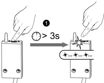
1 Press the receiver button for 3 seconds until the red LED flashes.
