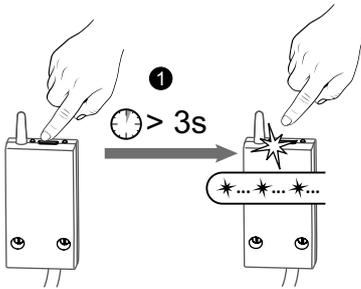
1 Press the receiver button for 3 seconds until the red LED flashes.
