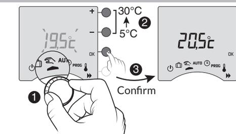
This mode is used to choose a set-point temperature that remains constant. Turn the selector dial to .
