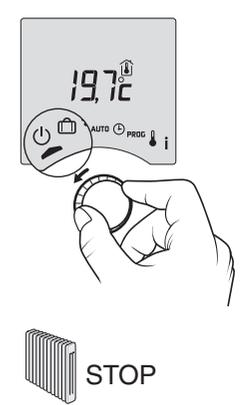
This mode is used to switch your heating installation off. Turn the selector dial to . In this mode, the device displays the room temperature.
