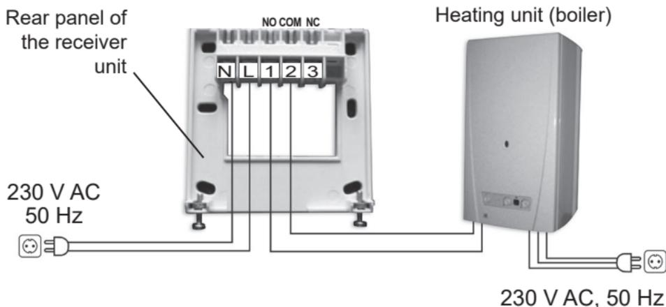
If you would like to operate an old boiler or any other device that has no connection points for thermostats, then the **1** (NO) and **2** (COM) connection points of the thermostat should be connected to the mains cable of the device, similarly as a switch would be connected, as shown in the figure below.
