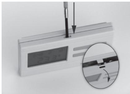
The battery compartment is in the inner side of the front panel of the housing. Insert 2 AA **alkaline** batteries (LR6 type) in accordance with the diagram in the battery compartment.
