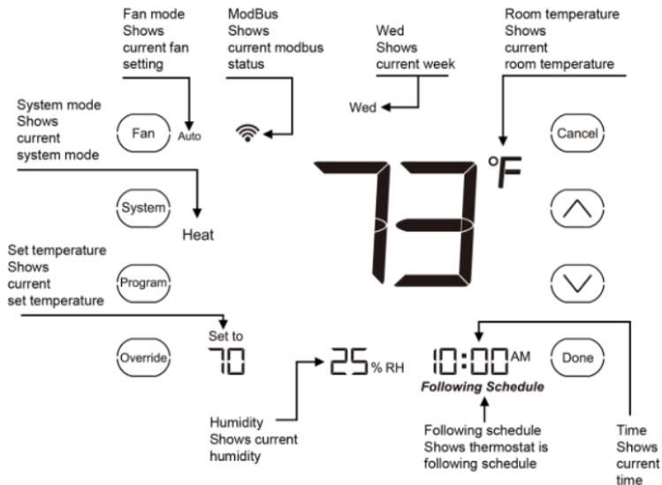
Figure 22. Thermostat display
