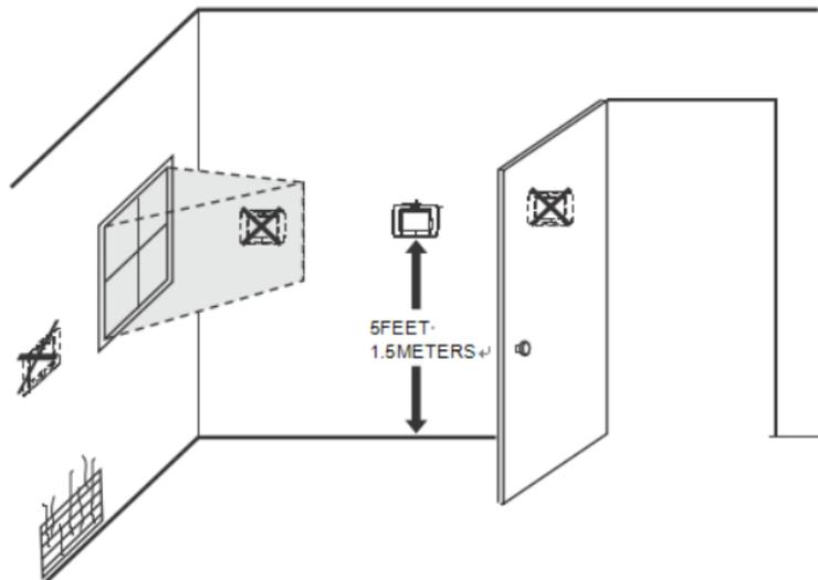
Figure 4. Selecting thermostat location
