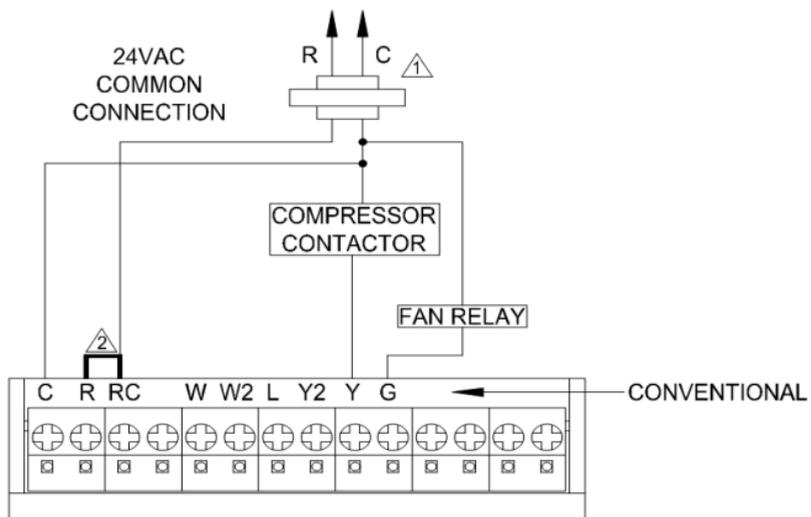
1. POWER SUPPLY. PROVIDE DISCONNECT MEANS AND OVERLOAD PROTECTION AS REQUIRED.
