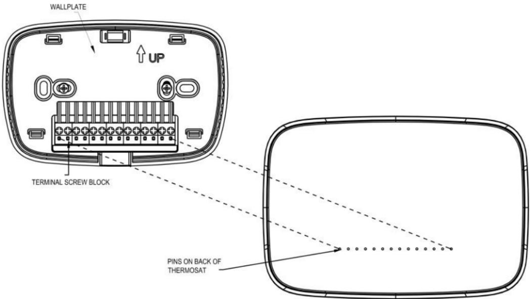
Figure 17. Mount thermostat to wall plate
