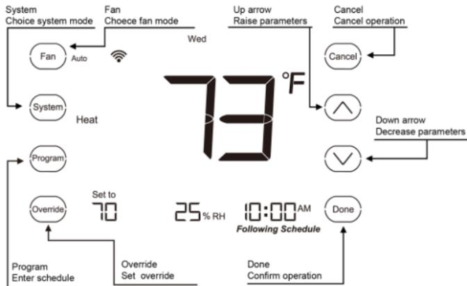
Figure 21. Thermostat keys
