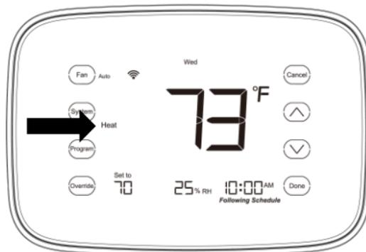
Figure 28. System mode is set to Heat
