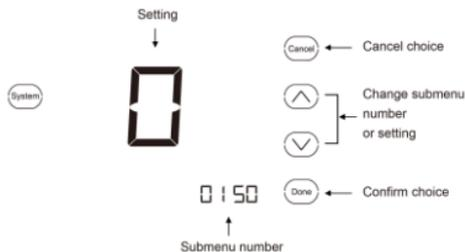
Figure 20. Arrow points to displayed submenu number and current setting
