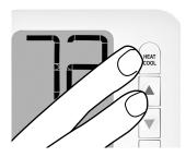
With thermostat powered, press System Mode button until **OFF** is underlined. After OFF mode is confirmed, press and hold BOTH the Menu and Up buttons for at least 5 seconds until the screen changes.
