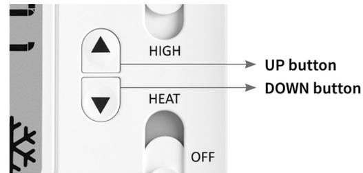
**UP / DOWN** = used for raising or lowering the target set temperature and selecting user options and settings in the display screen.
