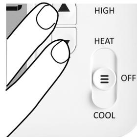
With thermostat powered, move System Mode switch to the OFF position. Press and hold BOTH Up and Down buttons for at least 5 seconds, until the screen changes.
