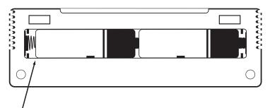
Insert 2 AA Alkaline batteries (included). High quality alkaline batteries are recommended.
