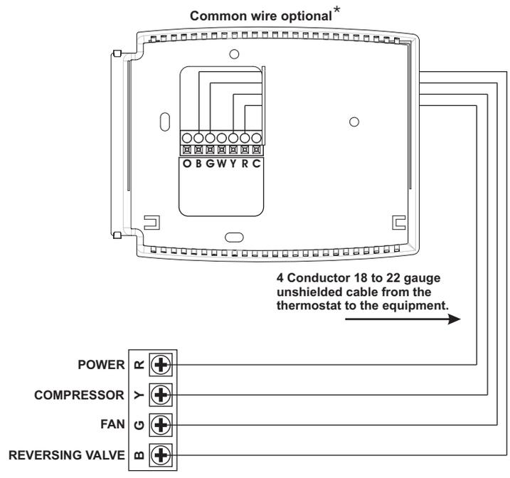
\* Common wire is optional in all installations. If a common wire is not used the thermostat must be powered by two AA alkaline batteries. These batteries must be replaced (page 11) each year or when the Low Battery indicator is displayed (page 3).
