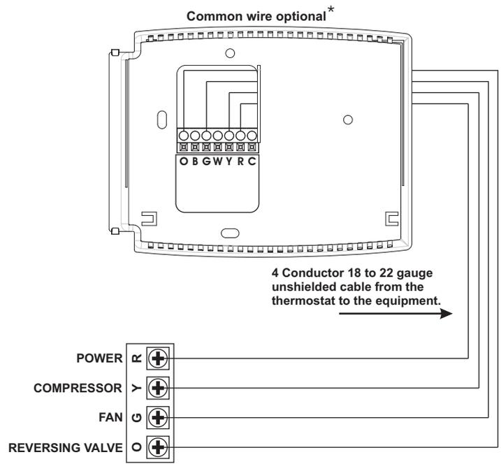
\* Common wire is optional in all installations. If a common wire is not used the thermostat must be powered by two AA alkaline batteries. These batteries must be replaced (page 11) each year or when the Low Battery indicator is displayed (page 3).
