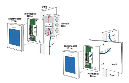
The Thermostat 560 operates a radiant floor heating system. The thermostat uses the built-in air temperature sensor.
