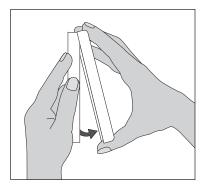
While holding the base section in one hand, pull the lower half of the display front towards you to pivot it away from the base.
